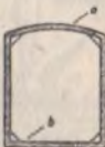
a. CAMBERED TOP OF THE BODY. b. FLAT BOTTOM OF THE BODY.
