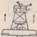
FRONT CONTROLS a FRONT STABILIZING SURFACE b FORWARD STABILIZER c FORWARD FIN d FRONT CONTROL SURFACE e FRONT ELEVATOR f FRONT RUDDER
