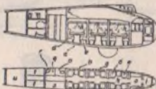
CLOSED PASSENGER CABIN a CABIN FLOOR b CABIN WALL c CABIN CEILING d PASSENGER'S SEAT e SEAT FACING FORWARD f SEAT FACING BACKWARD g COLLAPSIBLE WALL TABLE h WINDOW CURTAIN i GLASS WINDOW j CENTRAL GAWCWAY k COLLISION SPACE l PART BY PART TO LET m WASH ROOM n WASH BASIN o MAIL COMPARTMENT p LUGGAGE HOLD q RADIO CABIN
