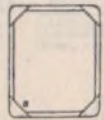
TRANSVERSE FRAME a GUSSET PLATE OF FRAME b MIDDLE PANEL c REAR PANEL
