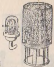
MULTI-LAMP BEACON WITH GLASS GLOBE BE SHOWN WITH COIL WITH (A) ONE LAMP IS FIRST; THE GLOBE (B) WITH (C) OTHER LAMP
