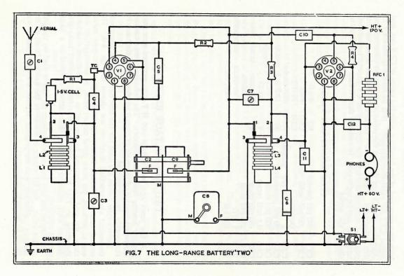
high frequency end of the band, i.e. with the vanes of C2-9 out, and adjust C3-7 for maximum strength. It is advisable to have C1 at *minimum*, and C8 just short of the point of oscillation when making this adjustment. Once set, C3-7 require no further attention. If powerful stations overlap, the capacity of C1 should be reduced until they can be separated. In extreme cases it may be necessary to shorten the aerial.
