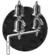
Twin lightning-arrestor and lead-in insulator with internal spark-gaps and lead-in fuses. Low-loss and adequately weather-proofed.
