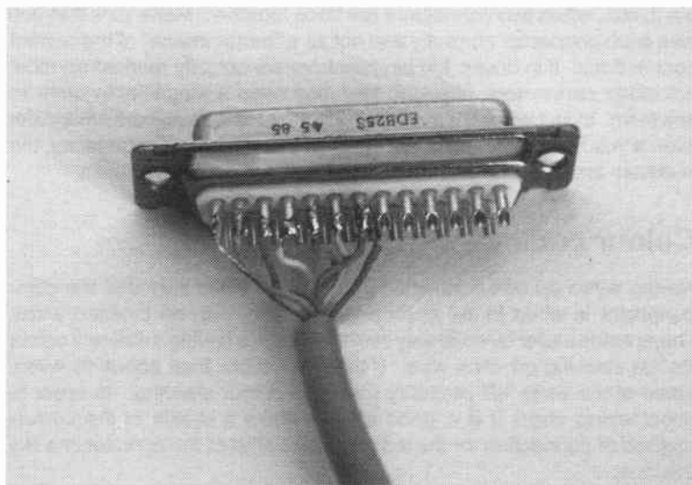
Fig.1.31 All the connections have been completed and the shell can now be fitted
