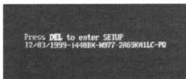
Fig.2.5 Pressing the Del key is the normal way into the BIOS Setup program
