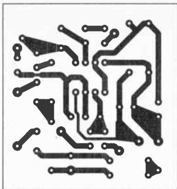
Fig. 3.7 Two-band active tone control PCB layout (actual size)
