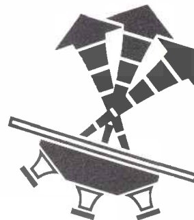
Unique wide-angle concave tweeter array — cuts through on-stage volume, eliminates beaming on-axis and muddy sound off-axis.
