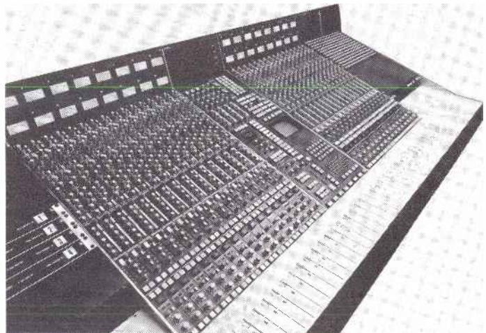
SSL SL4000 computer automated console.
