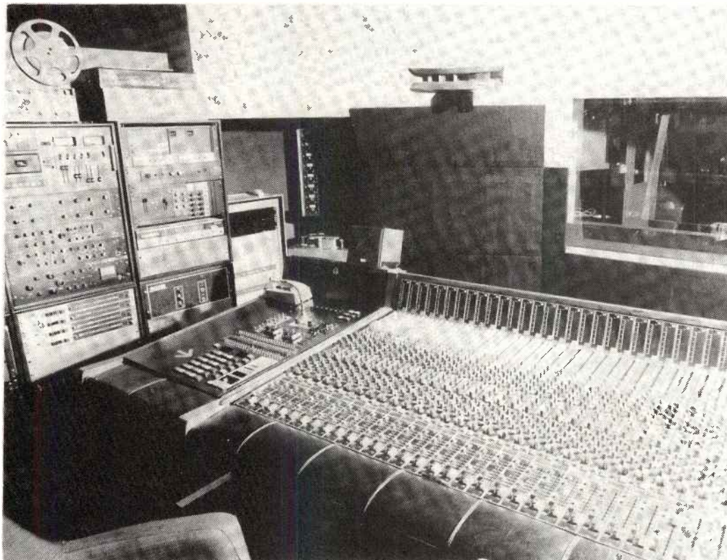
The recording console may be the one most important piece of equipment but ancillary gear (left of pic) plays a vital role, particularly if used with discrimination.
