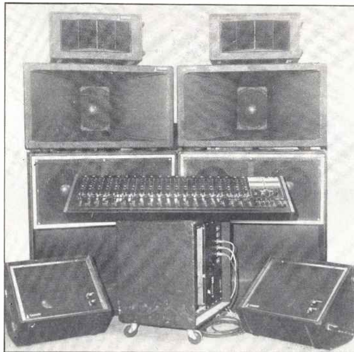
Canary P.A. with 2x12" horn-loaded reflex cabinets, 1x12" mid range exponential horns, 811B Altec sectoral horns and 2 '400' amps. The monitors each contain a 12" ATC plus a small RCF horn.
