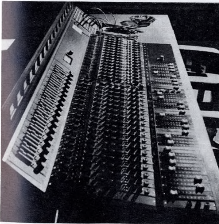
The Triad desk in the control room. It features 18 input and 16 output channels with full equalisation
