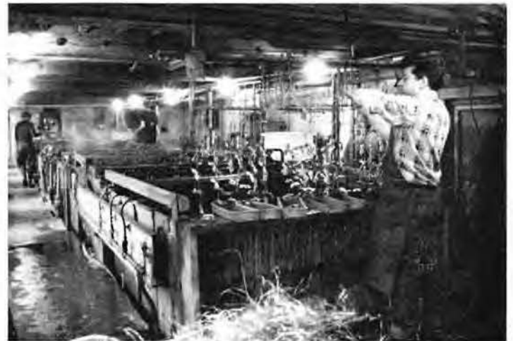
All the diamond chrome-finished accessories are plated at the specially-designed chroming plant in Canal Street. Before being passed through the chemical baths they are individually strung on copper wire.
