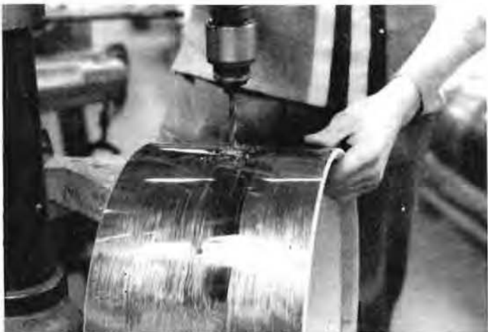
At Pullman Road, the finished drum shells are drilled for their fittings. The polyester finish has already been applied.
