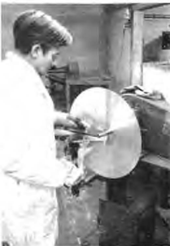
A cymbal being "spun" by a Premier craftsman in the metal works.
