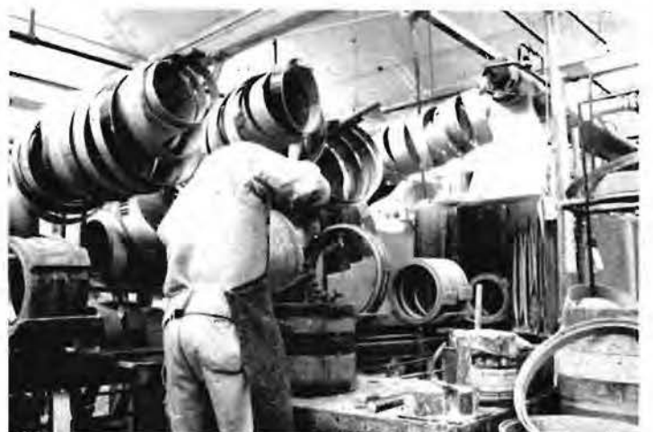
Here, the drum shells are glued, and take a slow trip round a circular conveyor belt. When they arrive back, they are removed and sent for finishing.
