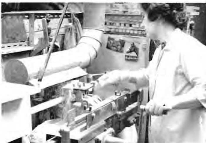
The lancewood or hickory drum sticks are planed down before being given their finish.
