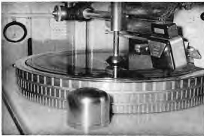
A close up of a disc-cutting machine producing a L.P. master.
