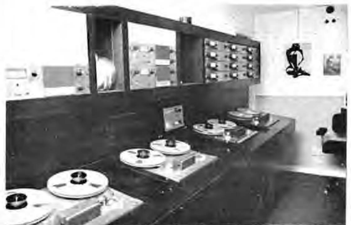
Trident's new Ampex 8-track tape machine, installed in a special tape machine room.
