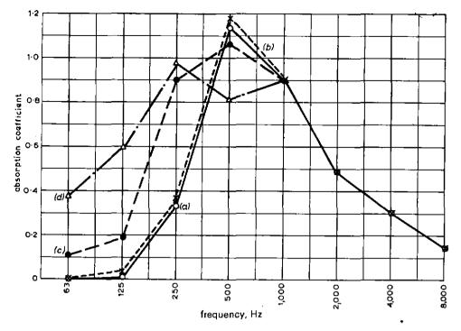
Fig. 3 — Absorption coefficient of Stillite Mineral Wool SR 10, thicknesses 1 in. (25 mm) and 2 in. (50 mm). 5% perforated hardboard cover
