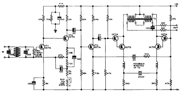
Fig. 7 — Line-receiving Amplifier: Circuit
