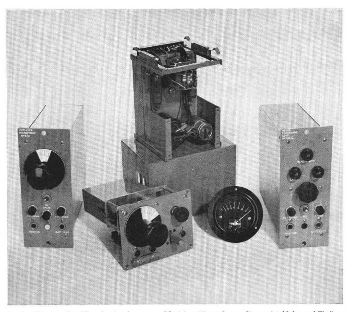
Fig. 8 — The group of amplifiers: the microphone pre-amplifier is in position at the rear of its associated fader panel. The line-receiving amplifier closely resembles the line-sending amplifier and only the latter is shown
