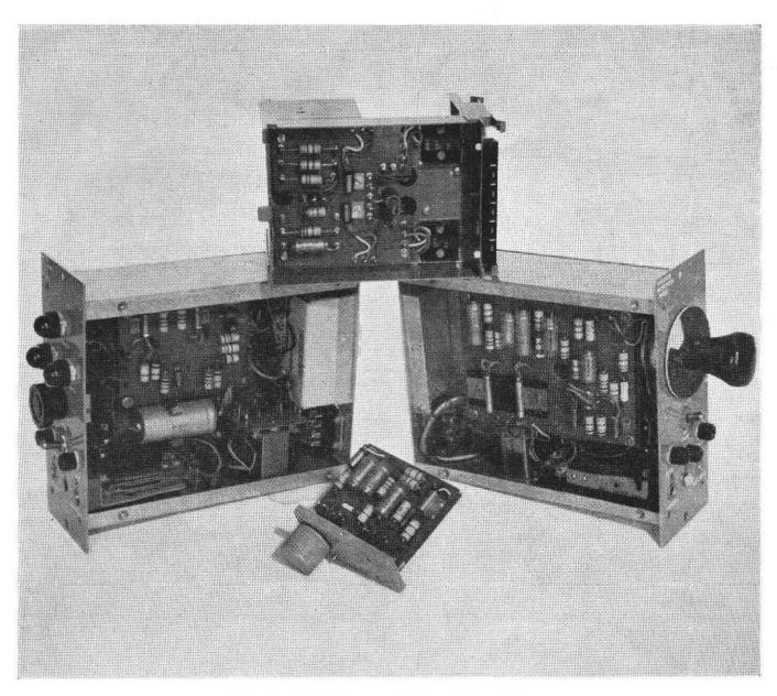
Fig. 9 — The interior construction of the amplifiers
