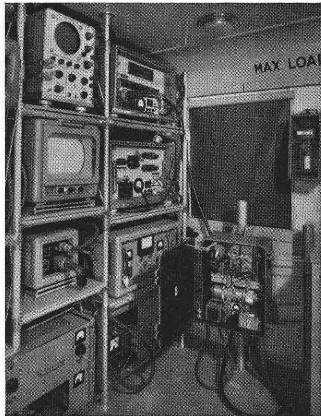
Fig. 5 — Band V receiver in the Roving Eye tender. Right-hand side, from top: 1st i.f. amplifier; 2nd discriminator. The cast case mounted on a scaffold tube is the head unit
