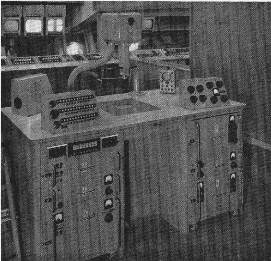
Fig. 17 — The Special Effects Control Desk in the Vision Control Room of Studio R1
