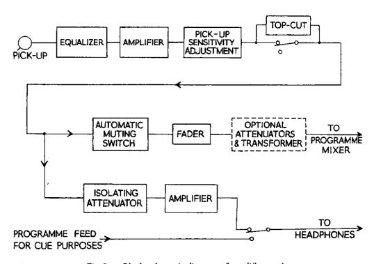
Fig. 8 - Block-schematic diagram of amplifier section
