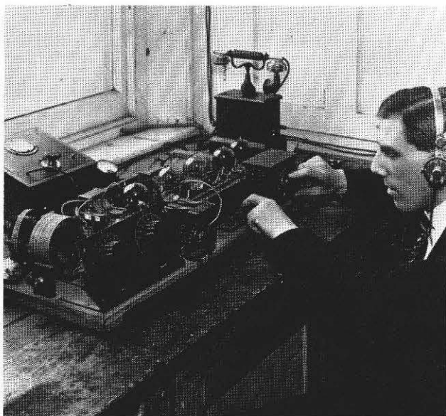
Fig. 24 Oxford and Cambridge boat race, 1927. One of the BBC receivers used for picking up the commentary from the launch Magician as she followed in the wake of the crews. Note that a regenerative detector – with no r.f. amplifier – followed by an audio amplifier, is used. The engineer is H. S. Walker of the Development Section.
