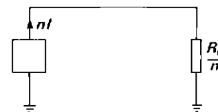
Fig. 9 The circuit of figure 8 further reduces to this, which is equivalent to a load of R_0/n on each transmitter.
