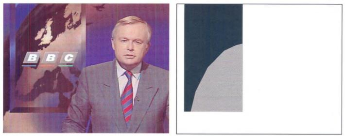
The photograph on the left shows presenter Martyn Lewis with graphic insert. On the right is the mask signal required to control the keying. The grey area allows CSO keying where the presenter's shoulder is likely to overlap the graphic. The black area forces the graphic through regardless of the backing and the white area forces the presenter and backing through.
