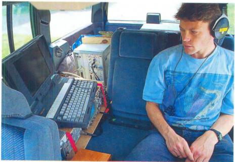
The interior of a newly-equipped vehicle for assessing experimental DAB coverage
