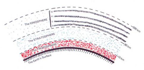
Fig 1: the earth's atmosphere showing the troposphere, the stratosphere and the D, E, F1 and F2 layers of the ionosphere
