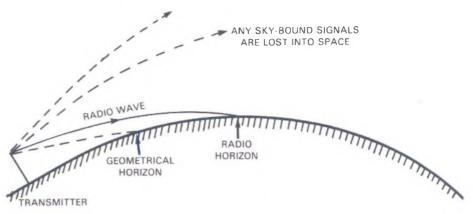
Fig 4: normal propagation of a vhf or uhf signal in the troposphere
