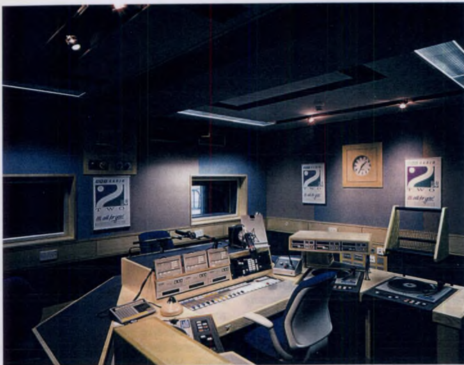
Suite 1G Studio: the fader tray can be covered with a neat ashwood panel when the studio is used in the non self-op mode
