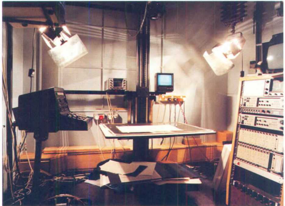
Rostrum cameras in the Electronic Caption Production Area (ECPA) at Television Centre.
