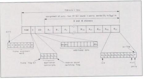
Fig. 1b: the NICAM 728 frame structure in more detail (stereo case)
