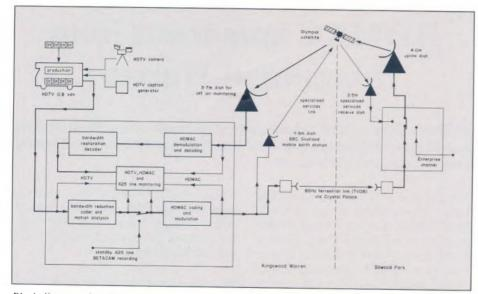
Block diagram of equipment used for HDMAC broadcasting tests from KW
