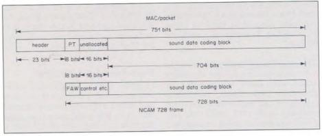
Fig. 1a: the frame structures of the MAC/packet and NICAM 728 systems
