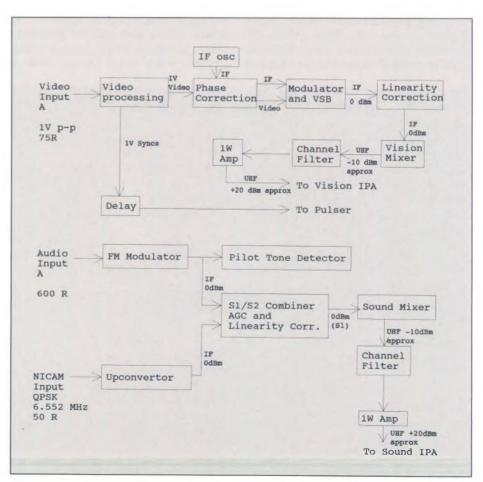
Block diagram of the new uhf transmitter system
