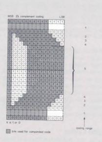
The diagram above shows the look-up table used in NICAM 728 to determine which 10-bit section of every 14-bit sample (within a given sound-coding block of thirty-two samples) will be transmitted. Note that three bits-per-block of thirty-two samples are needed to convey the range-code information to the decoders; in NICAM 728 these are conveyed using **Signalling-in-Parity** which is explained on page 17.
