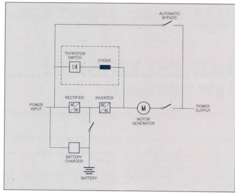
Fig. 1: the UPS system's block diagram
