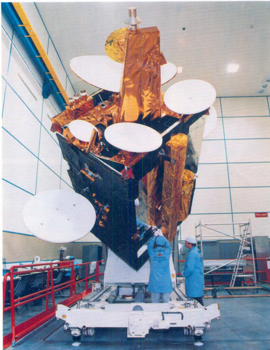
Olympus 1 Thermal Model (photo: British Aerospace)
