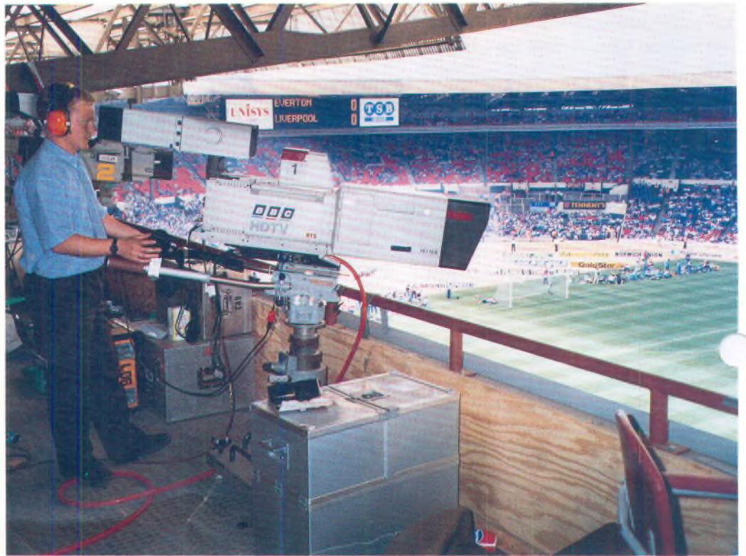
Recording the 1989 Cup Final at Wembley, in the 1250-line HDTV format
