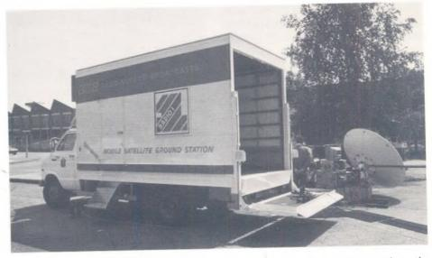
The transportable up-link, as rigged for tests at Concord Road in mid-June. In normal use, the dish aerial and associated equipment will sit on the tailgate of the OB vehicle shown.
