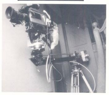
BBC Wales Mechanical Workshops have over the last year or so designed and manufactured two light weight O.B. crane arms for use with lightweight cameras, such as the Ikegami.
