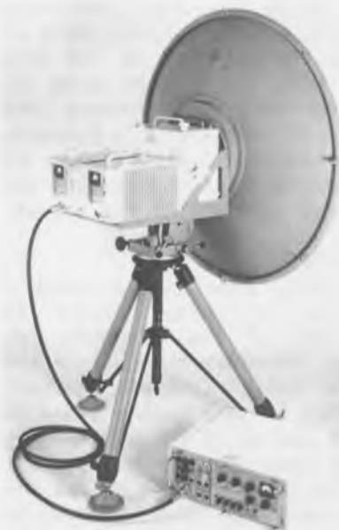
The new Continental Microwave link equipment.
