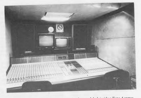
The Solid State Logic (SSL) computer-assisted control desk inside a Type A stereo control vehicle
