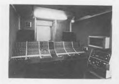
A Calrec 40-channel mixing desk inside a Type B stereo control vehicle Type B
