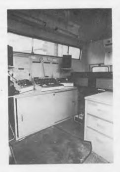
Interior of the digital recording vehicle. The two Mitsubishi/Telefunken recorders are at the rear (centre right).
