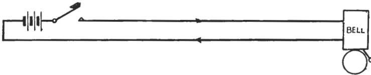
FIG. 6. SIMPLE BELL CIRCUIT
