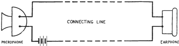
FIG. 32. A SIMPLE, ONE-WAY, TELEPHONE CIRCUIT
