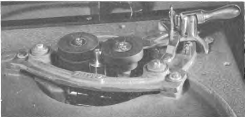
FIG. 44. PRESTO RECORDER 8N : DETAILS OF DRIVE AND SPEED-CHANGE MECHANISM
