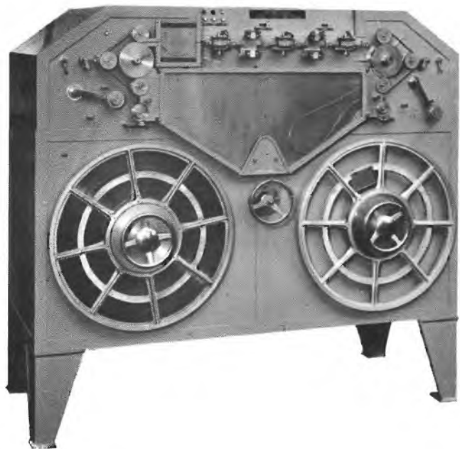
Marconi-Stille Tape Machines Used extensively for Overseas Services from 1934 onwards
