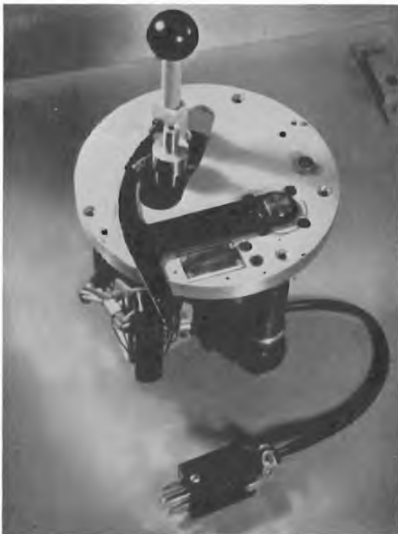
FIG. 91. REPRODUCING DESK DRD/1 ; TURNTABLE-DRIVE UNIT
