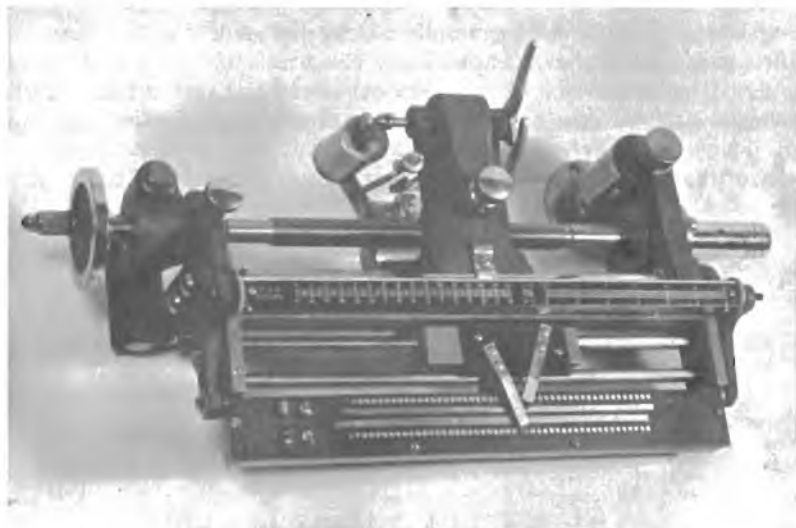
FIG. 48. PRESTO DISK RECORDER TRAVERSE UNIT TYPE-6N MACHINE Similar sliding contacts are fitted to the traverse unit on Type-8N machine
