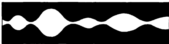
FIG. 116. VARIABLE-WIDTH SOUND TRACK
