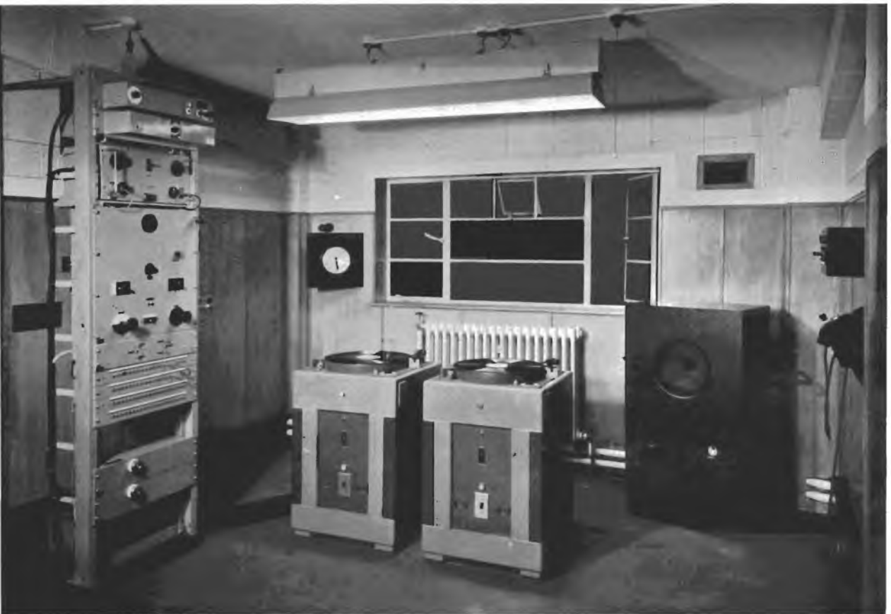
Disk Reproducing Channel, Aldenham, 1949 Presto two-speed reproducing machines, with E.M.I. Type-12 pickups and BBC auxiliary equipment
