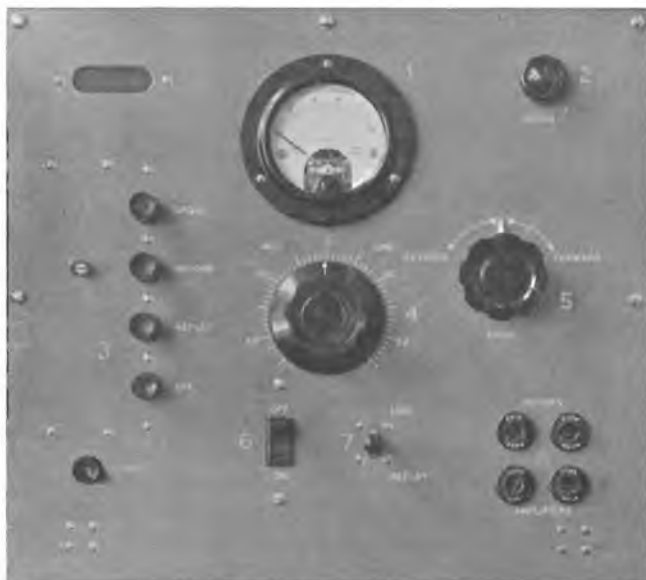
FIG. 114. E.M.I. MAGNETIC RECORDER : CONTROL PANEL
