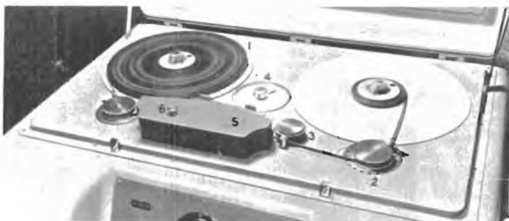
FIG. 112. E.M.I. MAGNETIC RECORDER : TOP PLATE SHOWING DETAILS OF TAPE DRIVE
