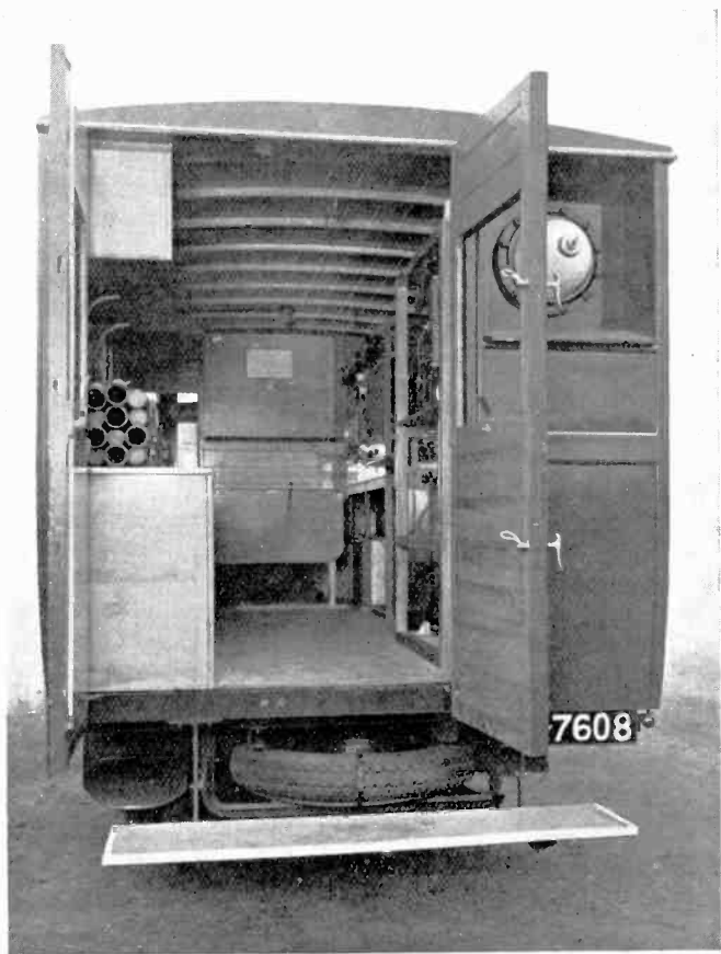
THE MOBILE TRANSMITTER USED FOR TESTING THE SUITABILITY OF A SITE
