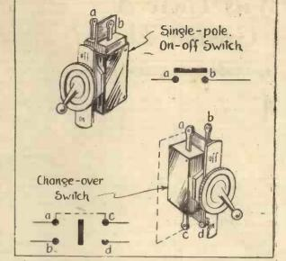
Fig. 1.—Two typical snap-type switches, a single-pole on-off and a change-over switch. Note the symbols beside them showing their mode of connection
