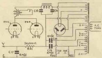
Fig. 3.—Showing the best arrangement for auto-biasing the output values working in parallel, so as to preserve the lower frequencies
