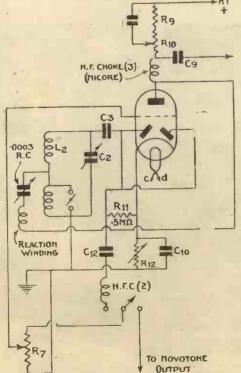
Fig. 5.—Showing how reaction may be introduced. Only the medium waves are affected
