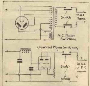
Fig. 3.—Two typical circuit applications for snap-type switches. Above is shown a double-pole an-off for mains set and below the same type of switch in a universal set where it is quite essential
