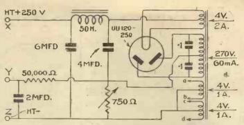
Fig. 2.—Circuit of the mains unit for the A.C. radio gramophone
