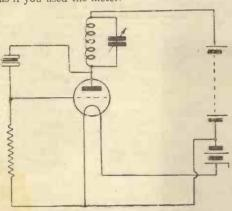
Fig. 1.—Quartz crystal across grid and anode of a valve
