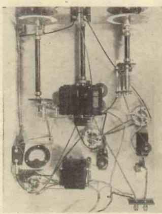
Plan view of the hook-up, showing how the all-wave coil and other components are arranged on the baseboard
