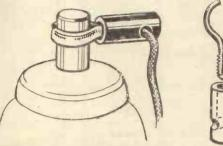
Clix anode connectors for use with modern valves having thimble tops
