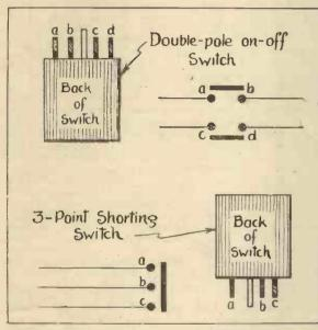
Fig. 2.—Back views of two more snap-type switches— at the top a double-pole on-off and below a three-point shorting switch for dual-range coils
