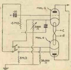
Fig. 4.—A switching arrangement by which an ML4 valve can be, if desired, added in parallel with the MHL4 in the second low-frequency stage, thus reducing both amplification and impedance when the ML4 is switched out of circuit; in this way practically no anode current is wasted
