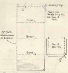
Fig. 1.—Layout of metal for square can—the top and bottom being separate pieces
