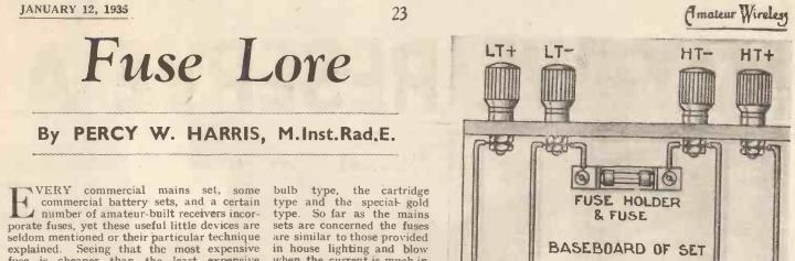
Typical fuse between high-tension negative and low-tension negative -fitted inside the set
