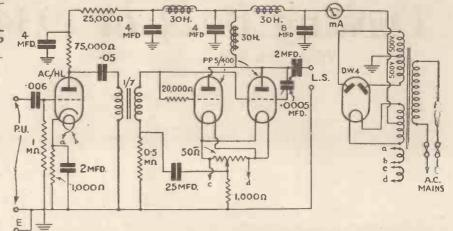
Fig. 5. Circuit of our A.C. amplifier, very simple considering it gives an output of II watts
