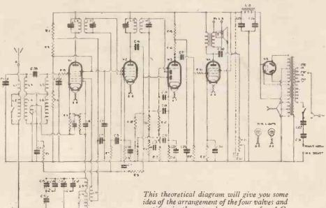
idea of the arrangement of the four valves and rectifier in the super-het sequence for A.C. mains operation
