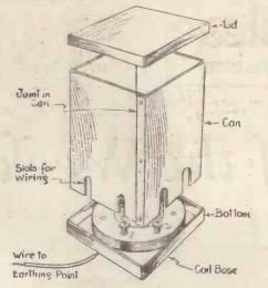
Fig. 4:—Completed can. It should be noted that the bottom piece is fixed underneath the coil base, with a wire gripped underneath for earthing to the chassis
