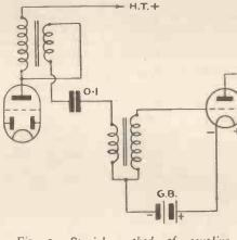
Fig. 2.-Special method of coupling between diode-triode and output valves
