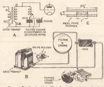
Fig. 3 .- Details of whistle filter for quality set : A, circuit ; B, diagrammatic connections ; C, dimensions of former
