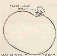
If a loop of wire is connected to a bulk it will light up brightly when brought near a transfermer
