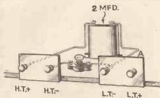
Fig. 2. Sometimes this fuse arrangement will "blow" every time the set is switched on, as explained in the article
