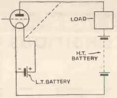
Fig. 1. Simple circuit showing current path in a valve circuit—following, it should be noted, the old convention
