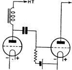
Fig. Choke-capacity 3. coupling
