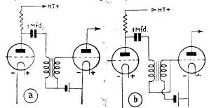
Figs. 5a and b.—Parallel-fed auto-transformer coupling
