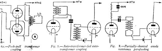
a coil winding offers an impedance to a transient signal, while the pure non-inductive resistance offers very little.
