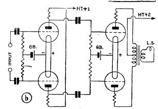
Fig. 6b.—Push-pull resistance coupling
