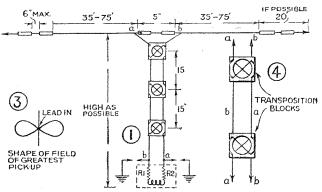
Fig. 1.—Horizontal doublet. Fig. 3.—Shape of field. Fig. 4.— Transposition blocks
