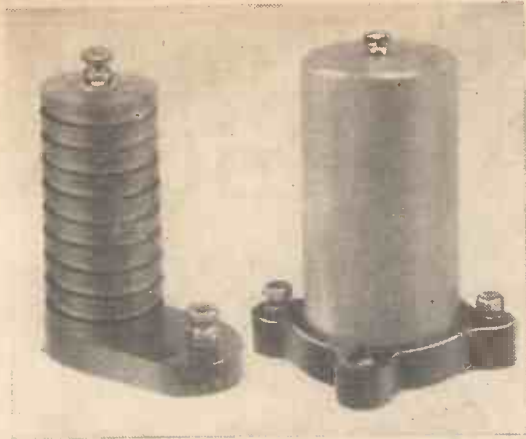
Two typical high-frequency chokes. That on the left is an ordinary slotted type, but on the right is one of the latest fully screened chokes
