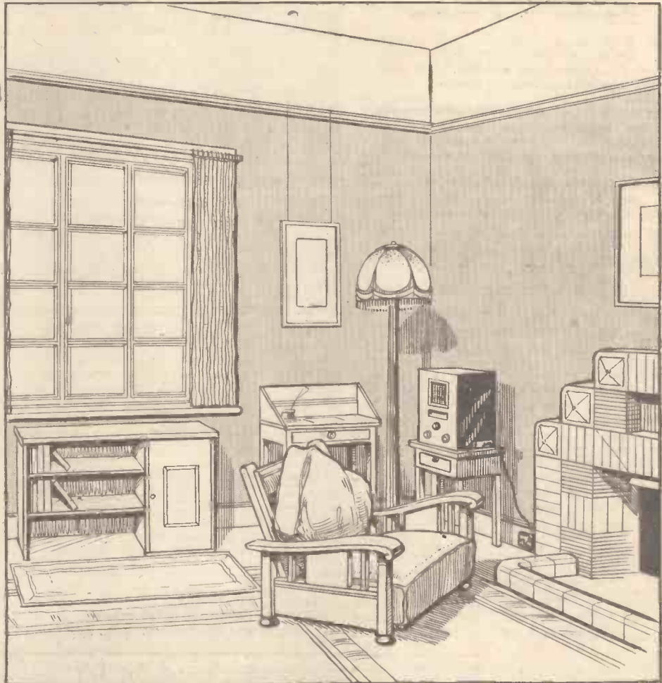
"An empty or barely furnished room in the modern style favours the reproduction of the higher frequencies . . . disappointing results are sometimes obtained when a set is taken home"
