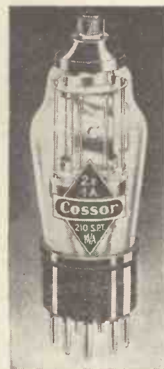
Of interest to battery users—the new Cossor 210 SPT battery high-frequency pentode
