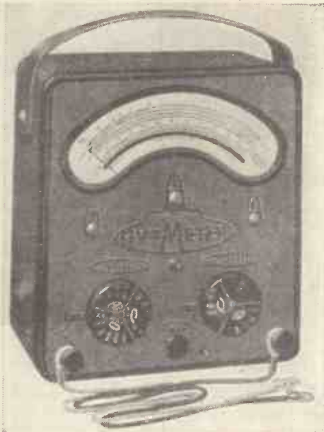
No Crusader can afford to be without some sort of testing gear. This new Avometer is a universal testing meter with no less than thirty-six different measuring ranges
