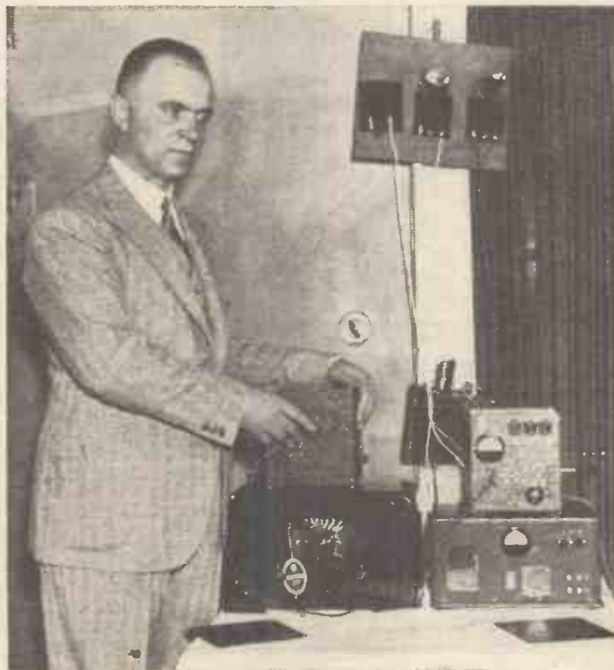
Wide World photo This gear is an automatic radio fire alarm developed in Berlin. By touching a switch a shrill alarm is put into operation
