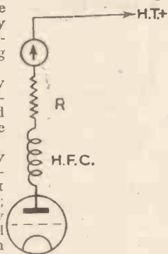
Fig. 2.—Milliammeter in the anode circuit of the detector valve for visual ganging
