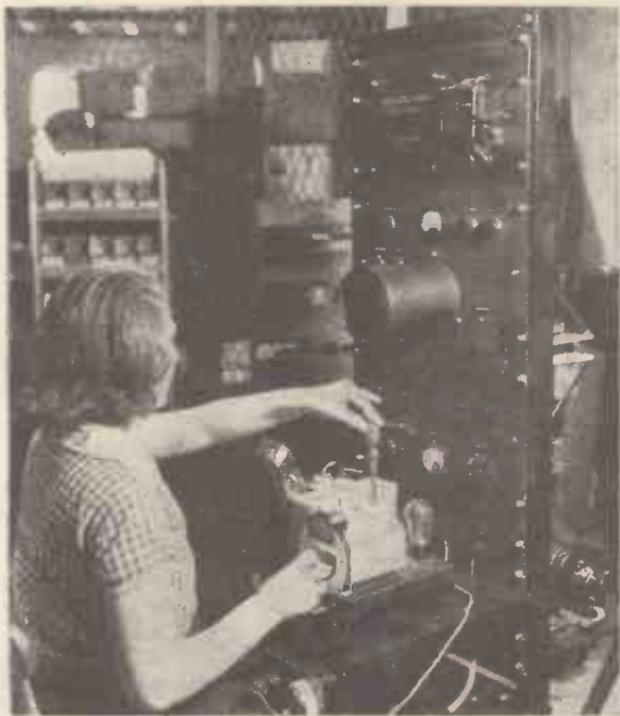
This test panel for ganging super-het receivers, makes use of a cathode-ray oscillograph
