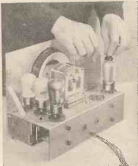
Connecting the flexible lead from the coil holder to the terminal on the top of the high-frequency pentode
