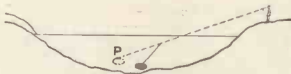
Fig. 1. How the eye sees a pebble in a pond. Due to the bending of the light rays the pebble appears nearer the surface
