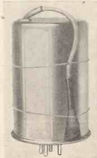
How the pigtail on an old coil can be strapped to the side of the can out of the way
