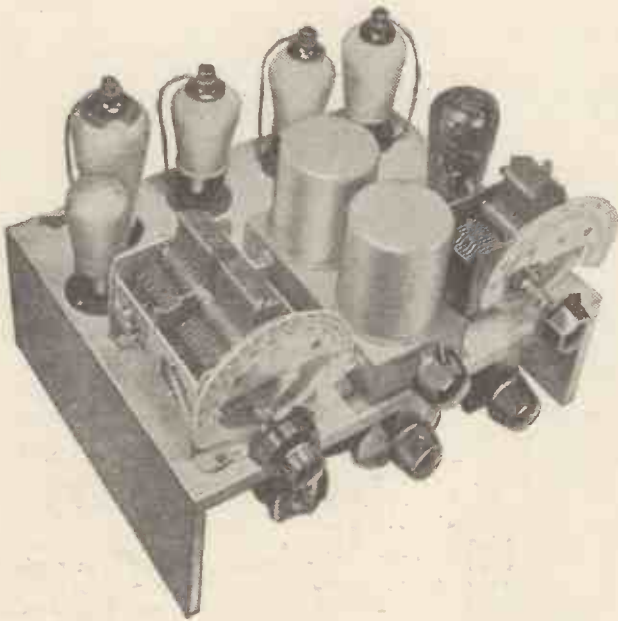
The completed 1934 Century Super, which takes advantage of the latest super-het technique
