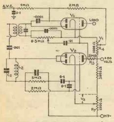
Fig. 3.—Two double-diode-triodes connected up to give quiet automatic volume control
