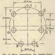
Fig. 4.-Base connections for double-diodetriode in the Marconi and Osram ranges
