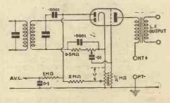
Fig. 2.—Double-diode-triode valve used in cir-cuit to give half-wave rectification and delayed automatic volume control
