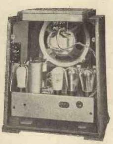
A rear view of one of the latest 4-valve super-hets-the Marconiphone model 272 -which represents all the latest technique in this class of receiver
