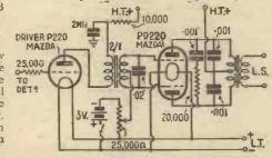
Fig. 3—The Mazda PD220 valve can be worked to advantage with this circuit. Note slight negative bias is needed
