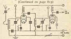
Fig. 7.—Suitable high-frequency-amplifier circuit for use with the automatic-volume-control circuits suggested in these pages
