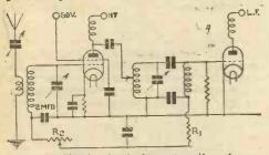
Fig. 1.—Simple circuit for automatic volume control, with resistance feeding back voltage from detector to control the amplification of the high-frequency valve
