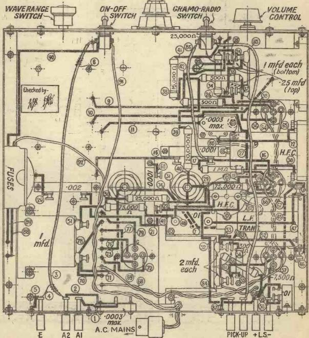
The more complicated part of the wiring is under the base, but it will be quite clear from this large-scale drawing. Full-size blueprints of both diagrams can be supplied for 1s. 6d. Details of upper side of the base are on page 808.
