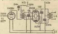
Fig. 2—For the Mullard PM2B valve, and similar valves when available in the Marconi and Osram ranges, this circuit is recommended
