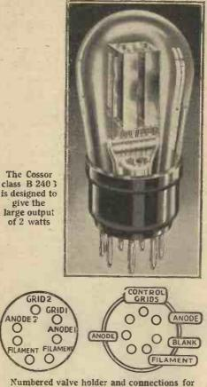
Numbered valve holder and connections for class B
