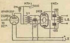
Fig. 1—Suggested circuit for use with either the Cossor 240B or the Ferranti HP2 valves
