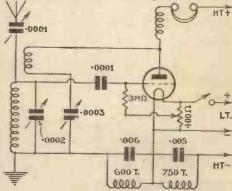
The main part of the circuit is that of a good short-wave one-valver. The Armstrong super coils, with their shunt condensers, are connected on the earth side of the grid circuit. Suitable condenser values to produce a quenching frequency either just audible or above the average audible range, are given in the accompanying article
