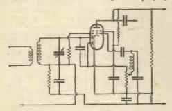
Fig. 5.--With the new Cossor DD/Pen valve automatic volume control is obtained with this simple circuit
