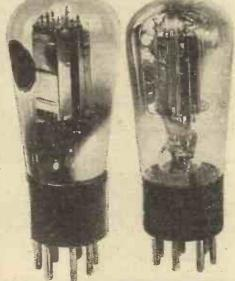
The Ferranti.HP2 and the Mazda PD220. In order still further to save current a small bias of .5-volt can be used with the Mazda PD220. The Ferranti HP2 is designed for high sensitivity
