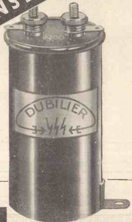
This is the Dubilier Type 9200 non-inductive Condenser which has been specially designed for by-pass purposes in H.F. circuits. It has a working voltage of 250 D.C. peak.
