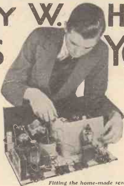
Fitting the home-made screen to the completed set
