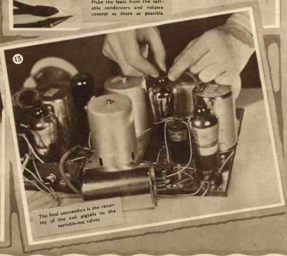
Refer to the full-size print before inserting the valves in their holders, as valve holders are also used for the coils
