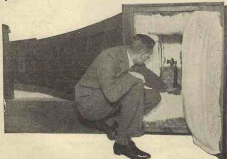
Putting 'phones through their paces! The baffle speaker idea is used by the Post Office engineers in testing 'phones for frequency response. The padded box acts in just the same way as a sound-lagged speaker baffle
