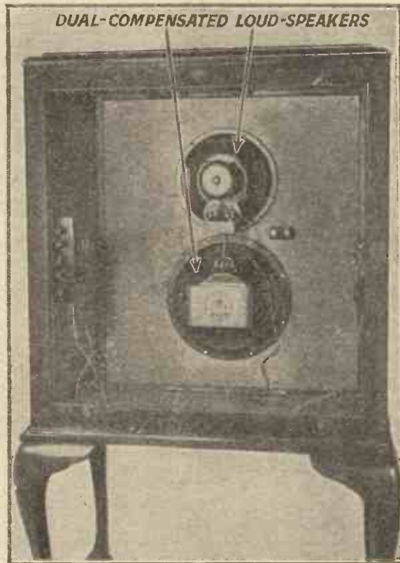
This photograph shows how the two compensated speakers are fixed on the one baffle
