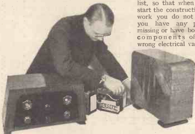
The final touch—connecting up the batteries. There is no reason why you should not build the "Wizard" in about a couple of hours
