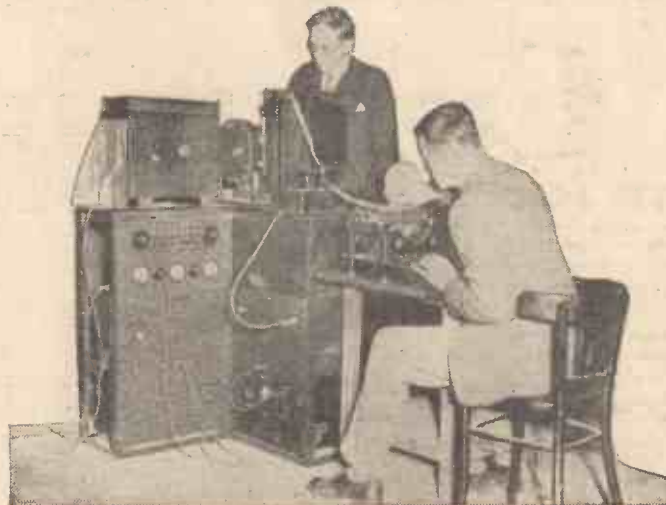
The operators at part of the new Marconi television apparatus which is being used for television tests between this country and Australia through the Chelmsford G2BS beam station. G5SW, the well-known short-waver, is also used for these television tests
