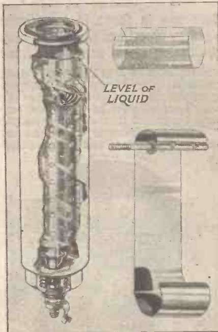
Chief constructional features of the Electrolytic condenser
