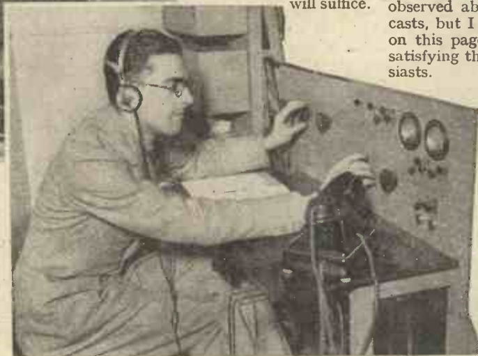
(Above) Controlling the mirror-drum scanning machine in the anteroom of the television studio. (Right) At the controls of the television mixing panel in the control room, where the photocell inputs are blended into the main amplifier input
