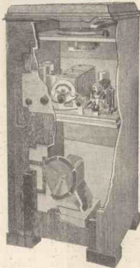
Used as a radio-gramophone, the “1932 Ether Searcher” in a console type cabinet and complete with gramophone equipment
