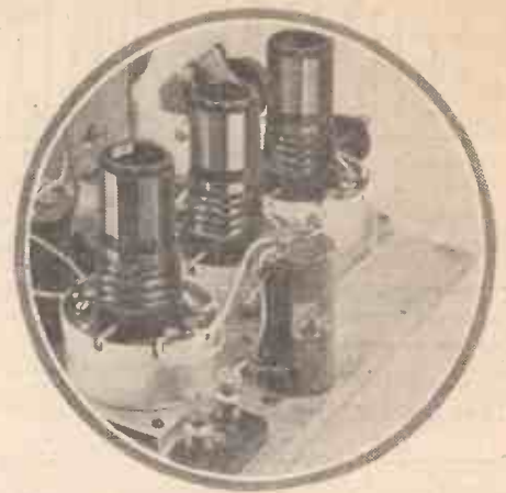
The "heart" of the "1932 Ether Searcher"—the band-pass tuner and coupling arrangements. The coils are shown without the screens
