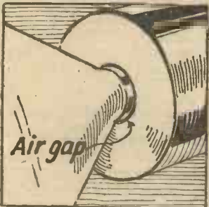
The air gap between the speech coil and the pot magnet of a moving coil speaker should be watched as chattering will be set up if it is not enough
