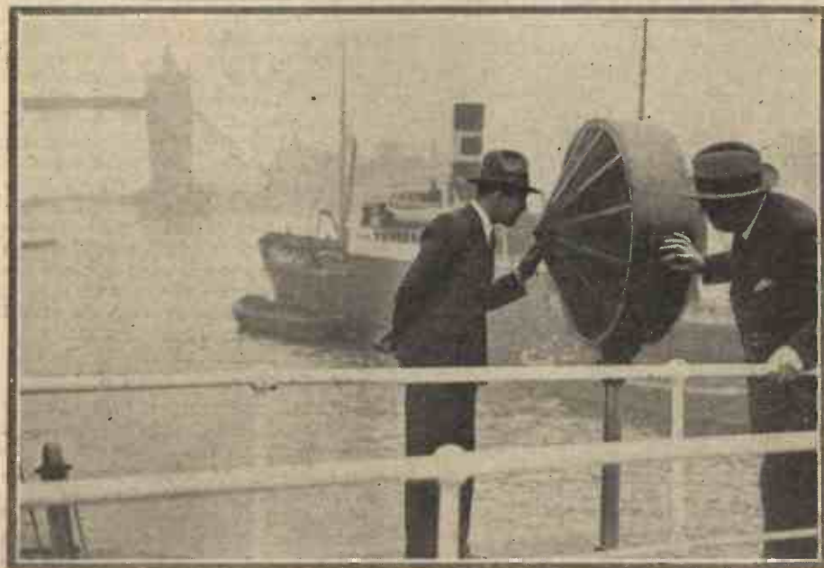
To make ships safe in fog. An official of the Port of London has designed this directional microphone to guide vessels by means of sound. It is being tried out on Thames shipping noises near the Tower Bridge and uses a wireless-type power amplifier
