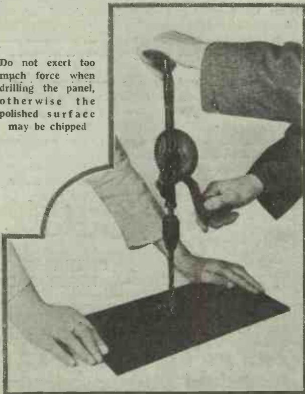
Keep the drill vertical. A willing helper holds the panel steady while drilling is in progress
