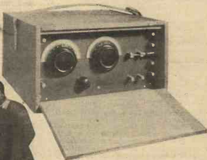
The one-valve short-wave set used with a standard three-valve R.C.-coupled amplifier for rebroadcasting in conjunction with the B.B.C.'s 100-watt transmitter
