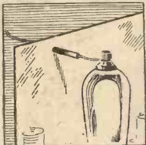
Watch wires passing through small holes in metal screens. A short length of thin rubber tubing slipped over the wire acts as extra protection
