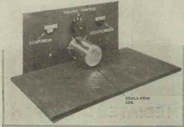
This shows the positions on the panel of the escutcheon plates, volume control, and oscillator coil
