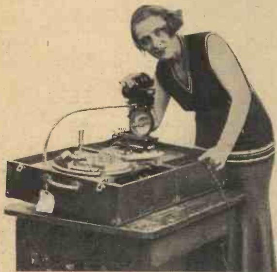
Making sound films in the home. The apparatus consists of an ordinary film camera, a miniature microphone, and a recording instrument resembling a portable gramophone. Recording or projecting is done with the same instrument, the camera or the projector being attached as required
