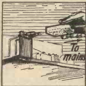
In the connection of mains apparatus the shielded sockets should be on the mains side and the projecting pins on the set or unit side
