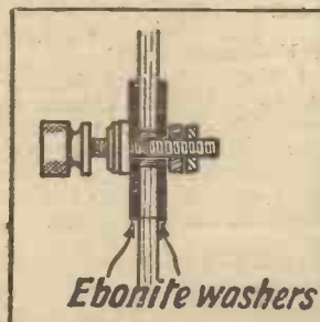
Terminals mounted on plywood panels may be insulated by allowing a clearance for the shank and having an ebonite washer on each side
