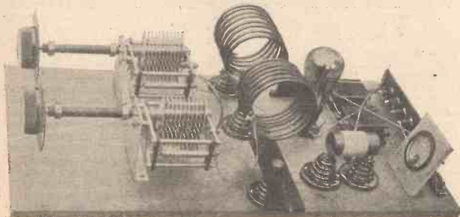
A single-valve short-wave transmitter which will be on the stand (No. 246) of the Radio Society of Great Britain at the forthcoming Exhibition
