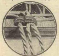
Terminals need not always be used. H.T., L.T. and G.B. leads can be twisted into groups and connected direct to the batteries the dials so that it does not touch the spindles of the panel parts.
