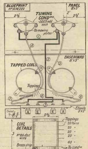
This plan view studied in conjunction with the wiring diagram will make the construction quite clear
