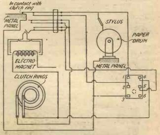
The Circuit Diagram of the Reproducer Unit
