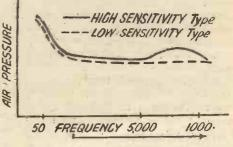
Fig. 2. Condenser Microphone Curves
