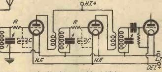
A grid resistance used for stabilising
