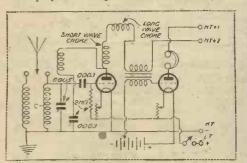
THE HOME-AND-ABROAD TWO.— This highly popular "A.W." receiver largely owes its popularity to its versatility. By means of three plug-in coils, the short, medium, and long waves can be brought in. The detector valve, to which Reinartz reaction is applied, is coupled to the L.F. valve through a transformer. Short- and long-wave chokes in series solved the problem of efficient choking for all waves.—Blueprint A.W. 77. Price 1/-.
