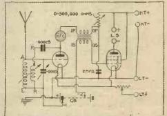
THE METEOR TWO.—Here is a set for the beginner. It is a very simple to build and easy to operate two-valver of exceptional power for only two valves. On a small indoor aerial in London it will bring in 5GB at full loud-speaker volume without interference from 2LO. It incorporates a simple all-wave tuner. Valves : detector and one L.F., transformer coupled. A good set with which to start.—Blueprint W.M. 114. Price 1/-.
