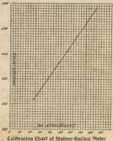
be obtained, and when located on the graph this point should, of course, fall on the straight line. The wavemeter can then be brought into use for checking the wavelengths of unknown stations.
