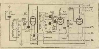
THE JAMES SPECIAL THREE.—This receiver, designed by Mr. W. James (our Research Consultant), has an exceptional performance. It incorporates new double-waveband aerial and H.F. coils—Mr. James's own design. Switching for the two wavebands is very simple. The circuit comprises screen-grid H.F., detector and transformer-coupled L.F. stages. Really inexpensive to build and run. The special coils can cheaply be made at home by the listener or can be bought.—Blueprint A.W. 156. Price 1/-.
