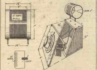
The Constructional Details of the Meter
