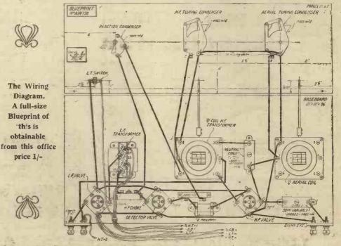
These are as follows: The aerial "Q" coil is placed on the left-hand side of the baseboard looking from the front and the split-primary "Q" coil is placed in the
